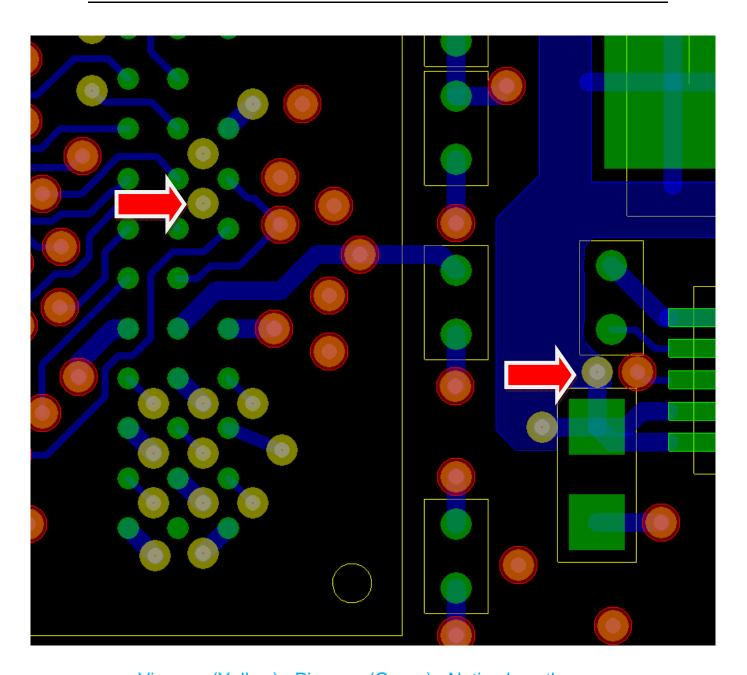
Vias are (Yellow). Pins are (Green). Notice how the soldermask openings (Red) are automatically reduced when they are close to a smt pad.
